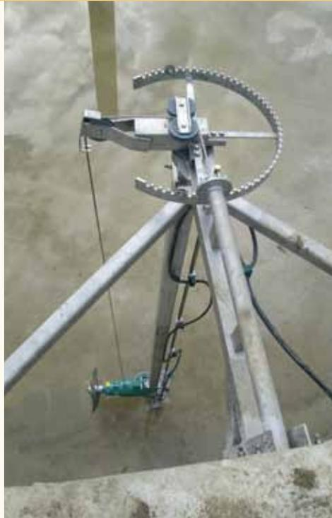
The guide mast with base frame is suitable for tanks with a depths of 39' and includes wall support inside and outside the tank, gastight cable- and rope lead throughs, external rope winch with a  $\varnothing$  0.3" ss316 rope and a handwheel for the vertical adjustment of the agitator.
